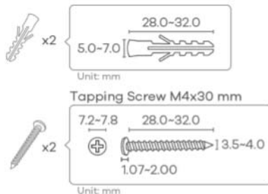
Figure 4 Screw Specifications
