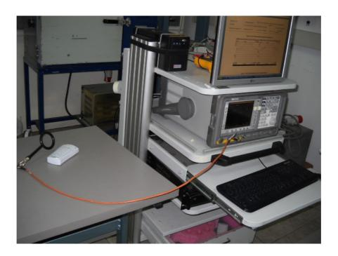
Photograph No.9 Setup for band edge emissions and hopping parameters measurements
