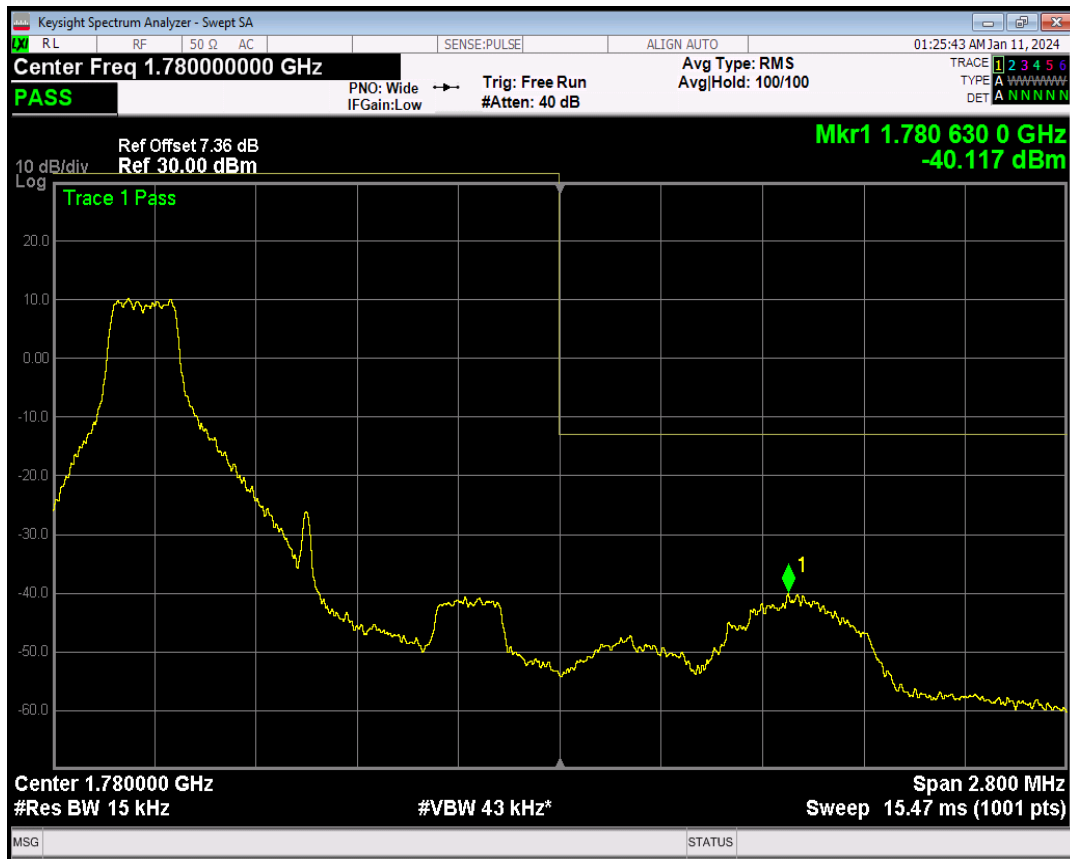
Band66 16QAM BW=1.4MHz Channel=132665 RB Size=1 Position=#Max
