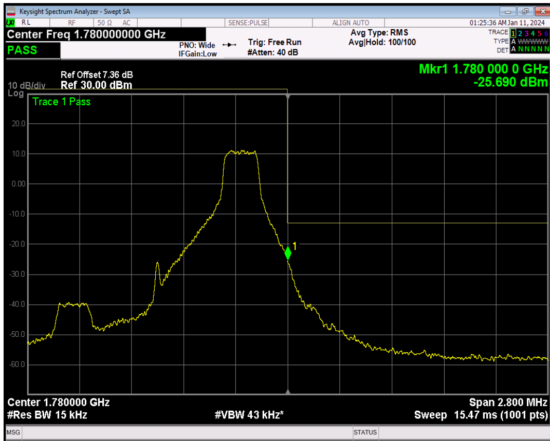
Band66 QPSK BW=1.4MHz Channel=132665 RB Size=6 Position=#0
