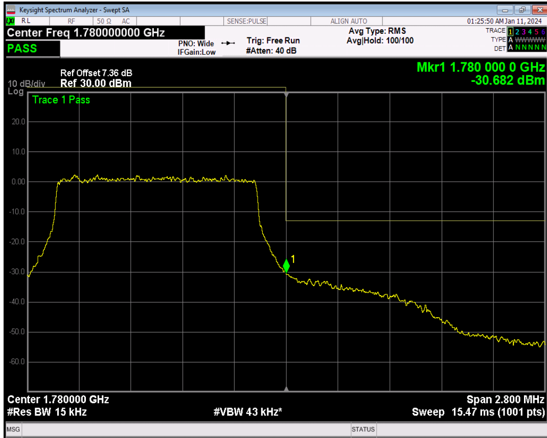
Band66 QPSK BW=3MHz Channel=131987 RB Size=1 Position=#0
