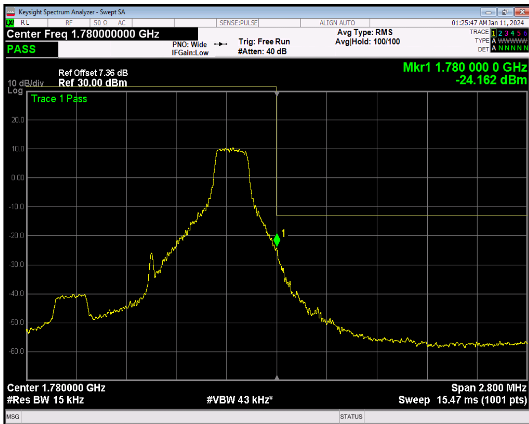
Band66 16QAM BW=1.4MHz Channel=132665 RB Size=6 Position=#0
