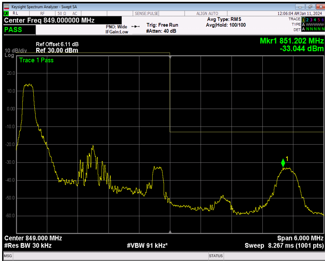
Band5 16QAM BW=3MHz Channel=20635 RB Size=1 Position=#Max
