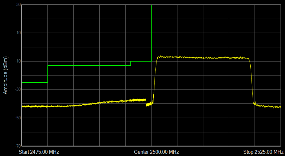
Band7 QPSK BW=20MHz Channel=20850 RB Size=100 Position=#0
