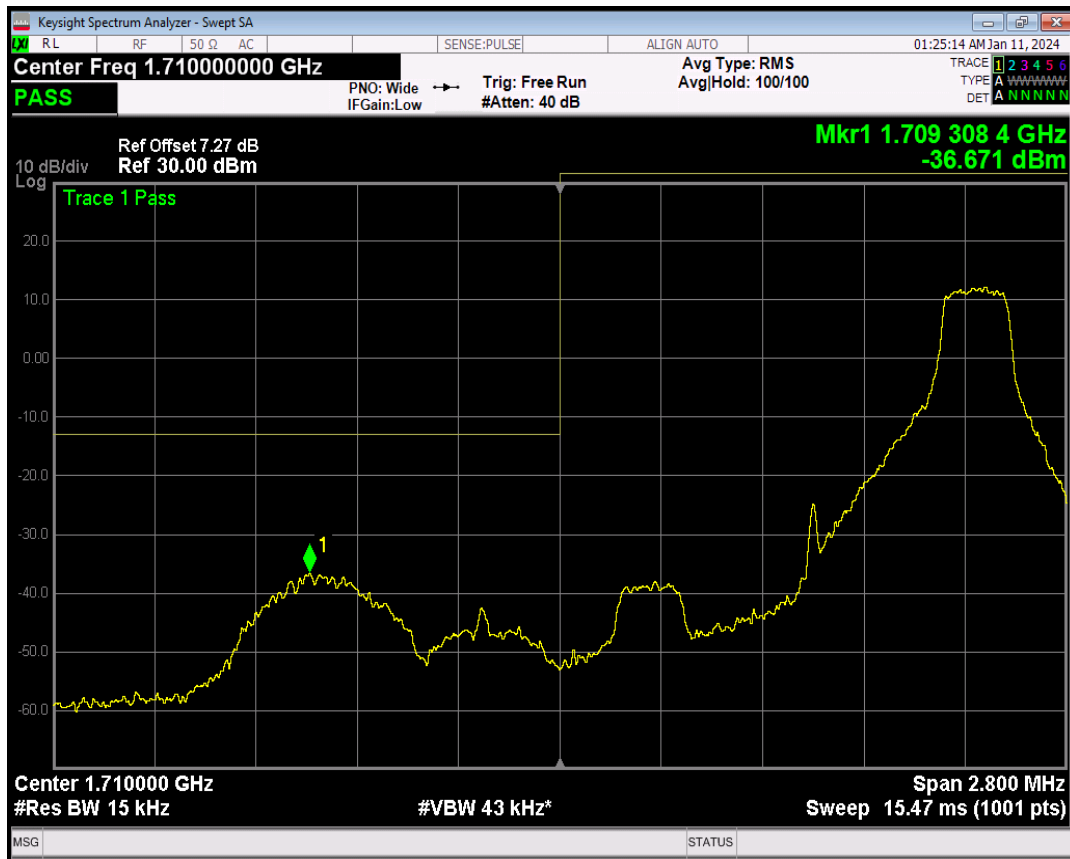
Band66 QPSK BW=1.4MHz Channel=131979 RB Size=6 Position=#0
