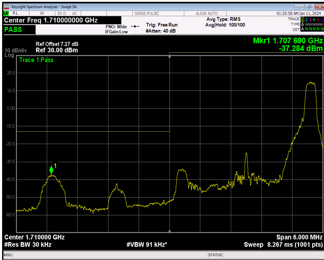
Band66 QPSK BW=3MHz Channel=131987 RB Size=15 Position=#0
