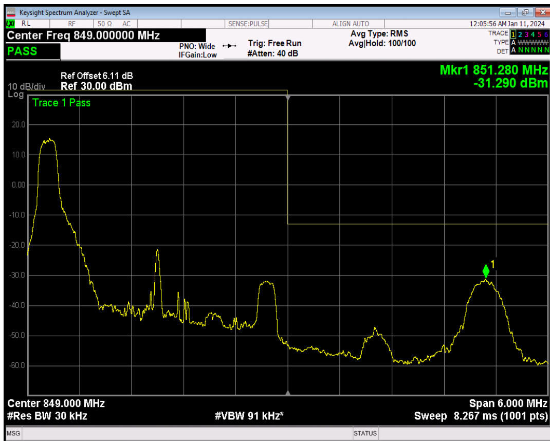
Band5 QPSK BW=3MHz Channel=20635 RB Size=1 Position=#Max
