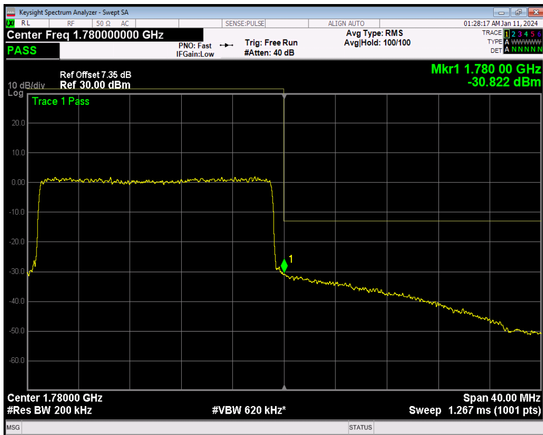
Band66 16QAM BW=20MHz Channel=132572 RB Size=1 Position=#0
