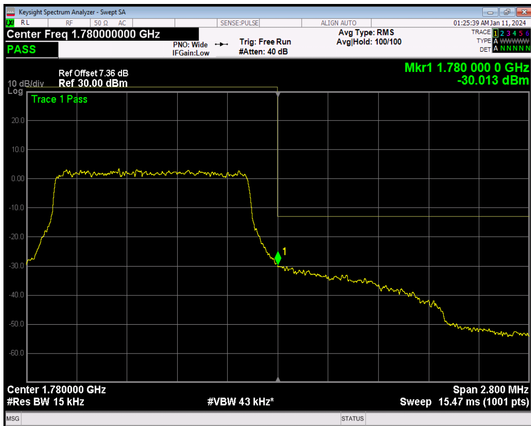
Band66 16QAM BW=1.4MHz Channel=132665 RB Size=1 Position=#0
