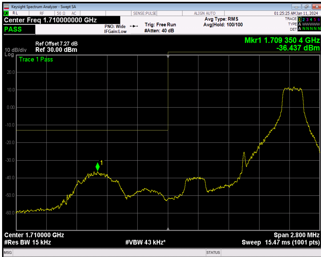
Band66 16QAM BW=1.4MHz Channel=131979 RB Size=6 Position=#0
