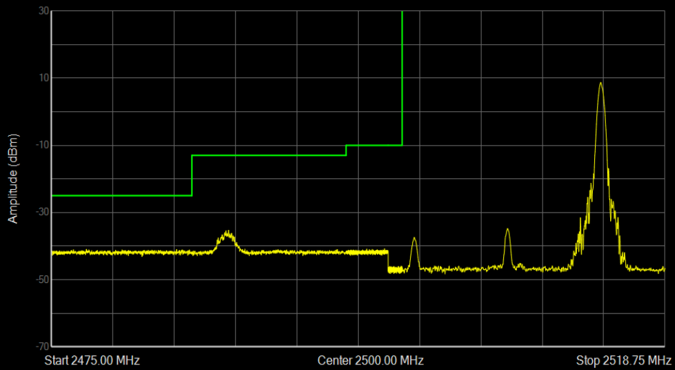
Band7 16QAM BW=15MHz Channel=20825 RB Size=1 Position=#Max
