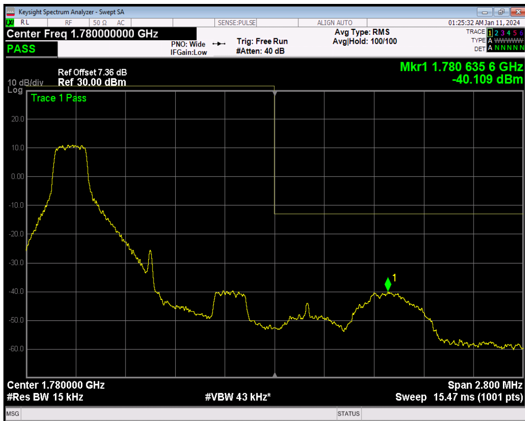
Band66 QPSK BW=1.4MHz Channel=132665 RB Size=1 Position=#Max
