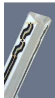
Figure 4.2 Probe Thick-Film Technique
