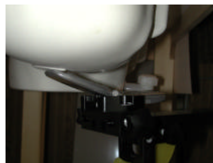
Figure 15.2 Right Head SAR Test Setup -- Ear / 15° Tilt Position --
