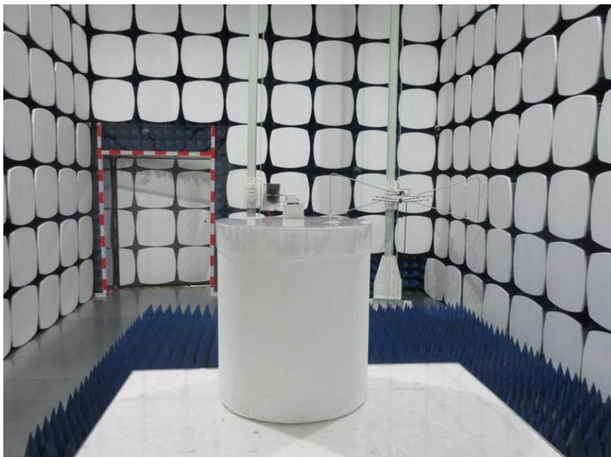
1.3 Radiated Spurious Emissions Test Setup
