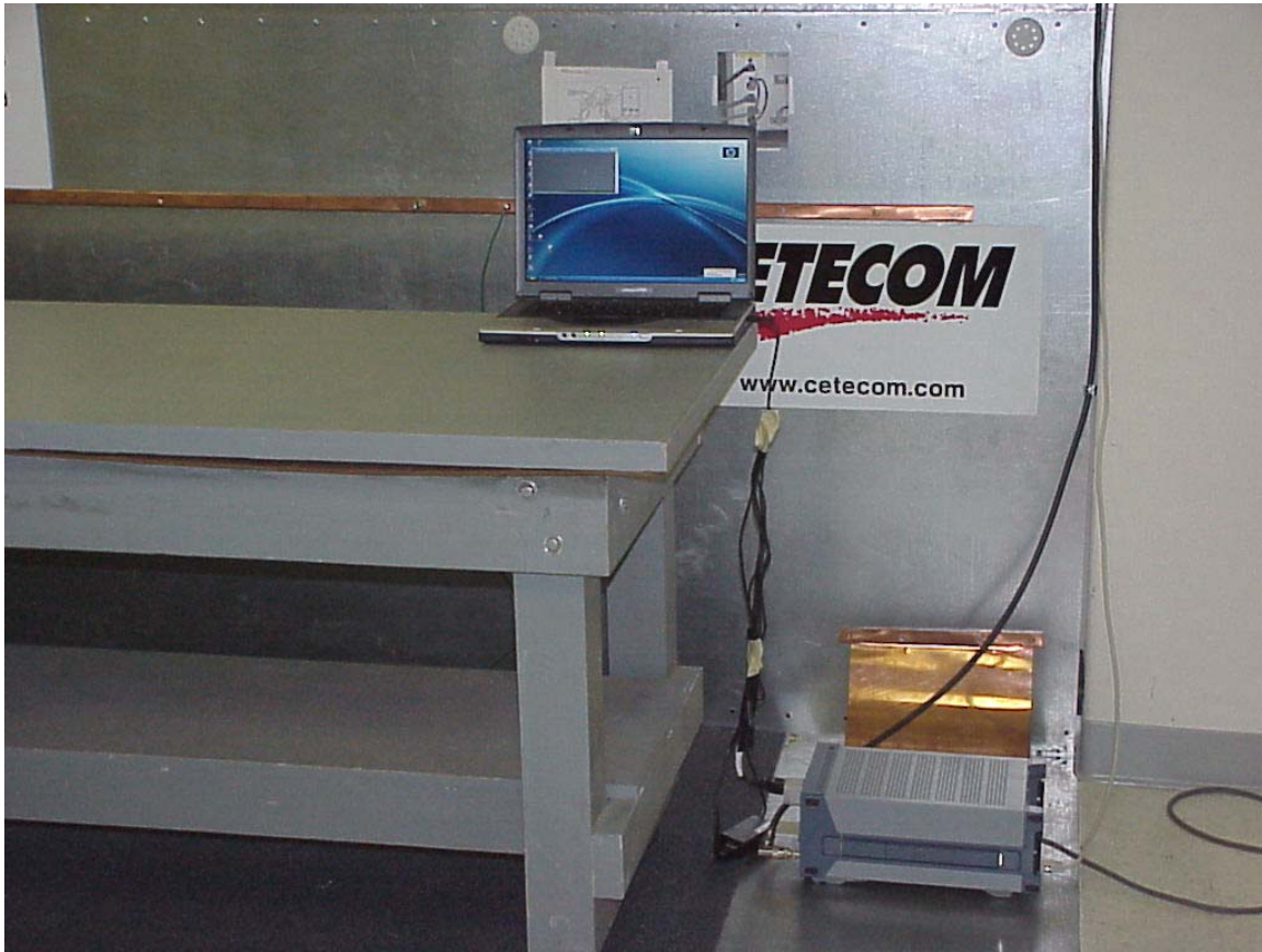
Test set-up – AC Line conducted emissions
