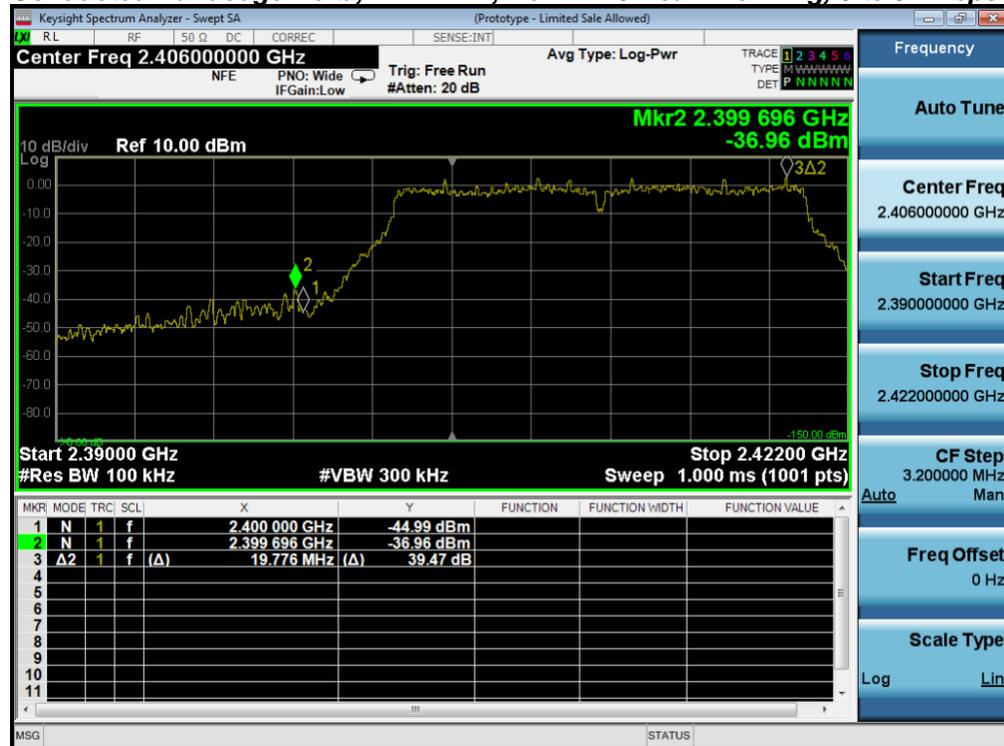
**Conducted Bandedge Delta, 2462 MHz, HT/VHT20, M0 to M15**
