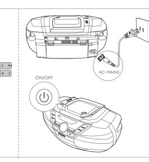
EN To operate this device, you can use either batteries (type: R-20 or D-cells) or AC power.
