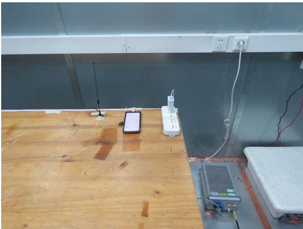
Picture 2 Conducted Emission Test Setup
