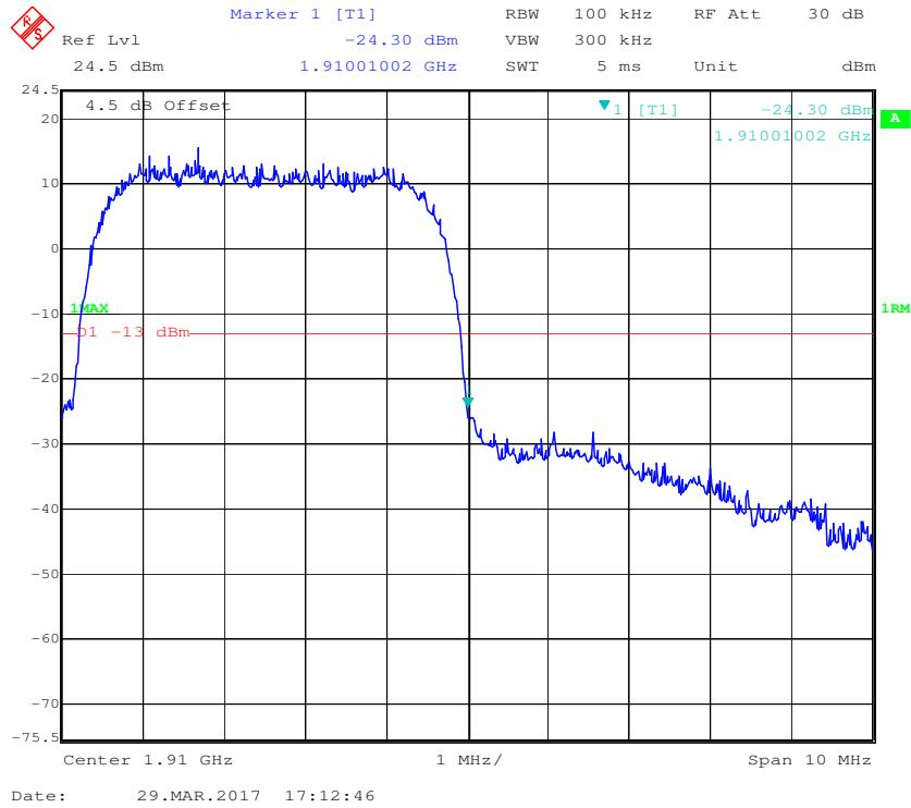
**PCS Band, Left Band Edge for HSUPA (BPSK) Mode**
