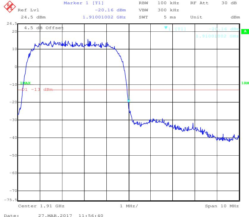
**PCS Band, Left Band Edge for HSDPA (16QAM) Mode**
