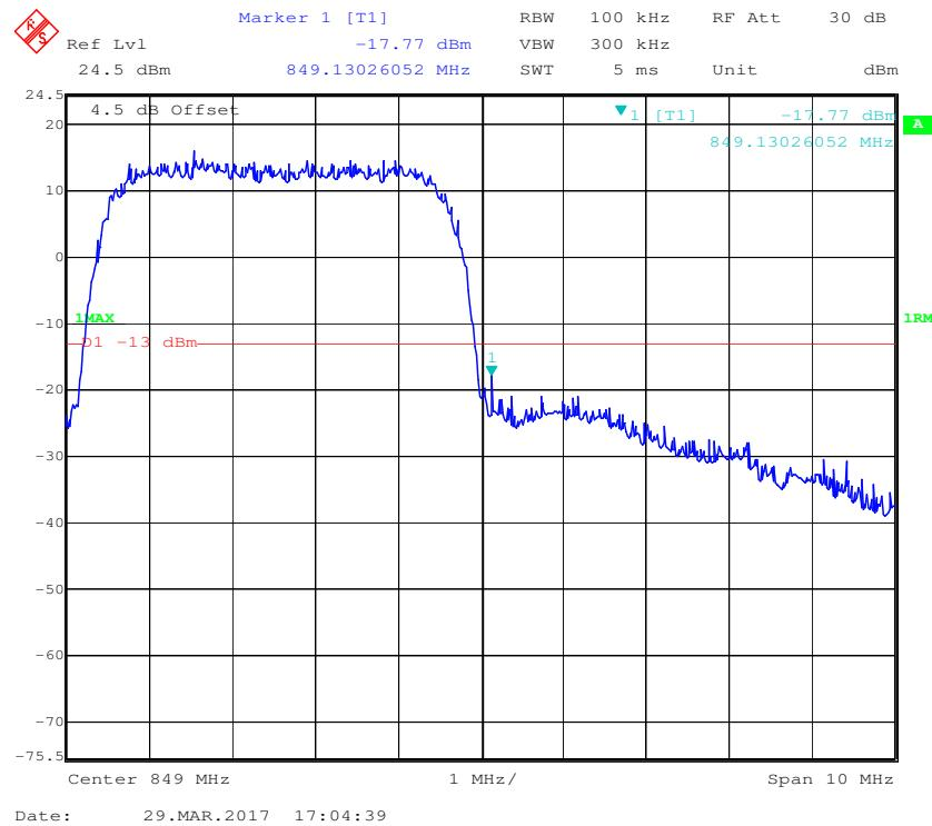
**PCS Band, Left Band Edge for GSM (GMSK) Mode**
