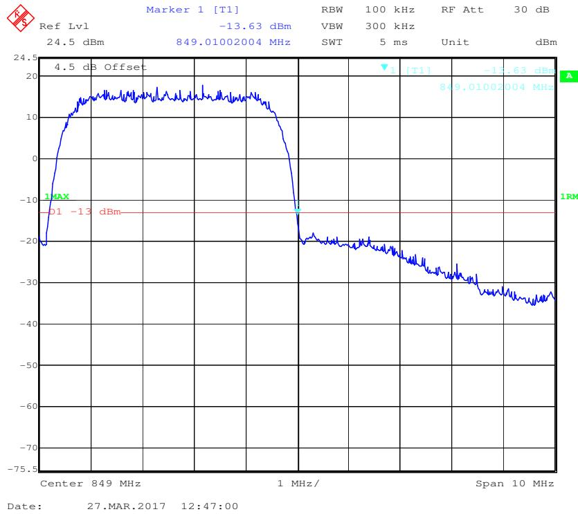
**Cellular Band, Left Band Edge for HSDPA (16QAM) Mode**
