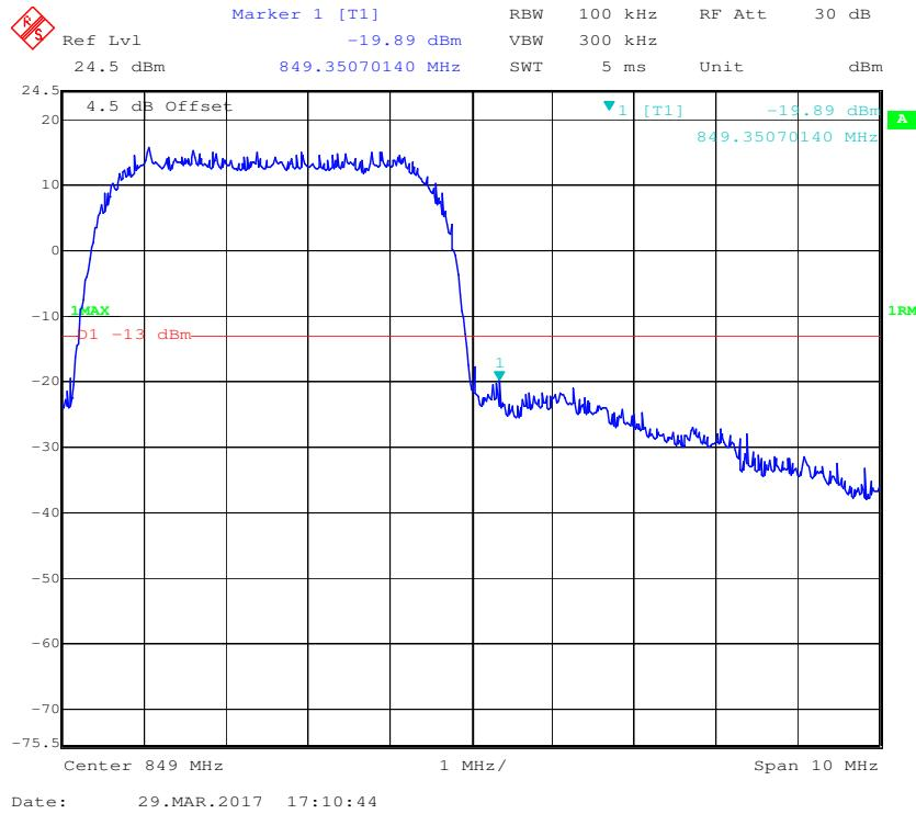
**Cellular Band, Left Band Edge for HSUPA (BPSK) Mode**
