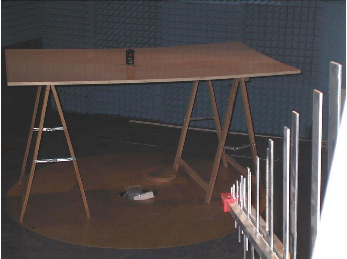
Picture RE/3 Radiated Emission Setup 30MHz-1000MHz
