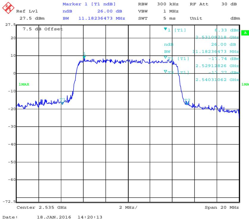
**QPSK (15.0 MHz) - 26 dB Bandwidth, Middle channel**
