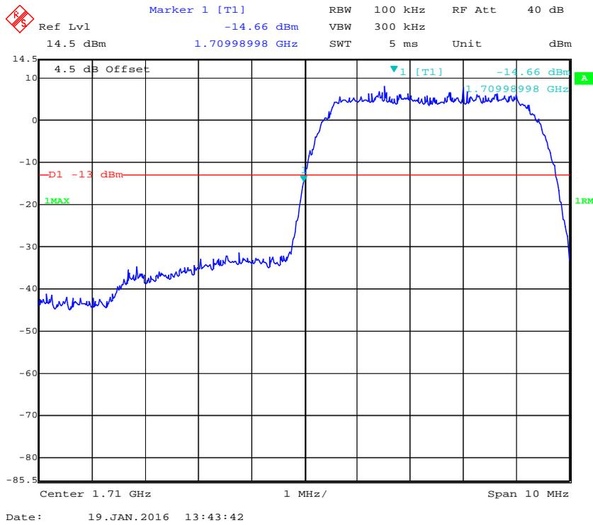
**AWS Band, Right Band Edge for HSUPA (BPSK) Mode**
