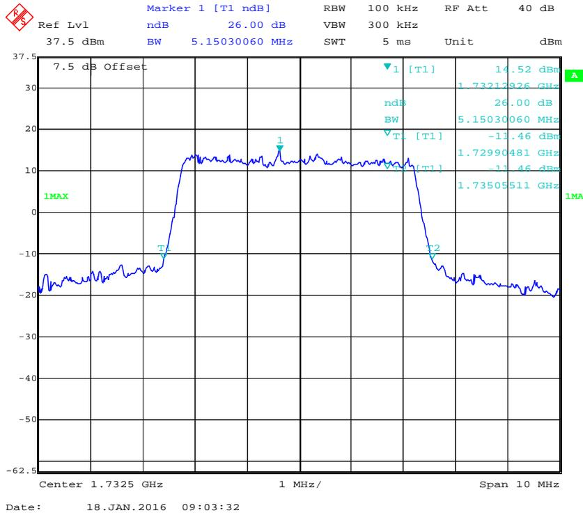
**16-QAM (5.0 MHz) - 26 dB Bandwidth, Middle channel**
