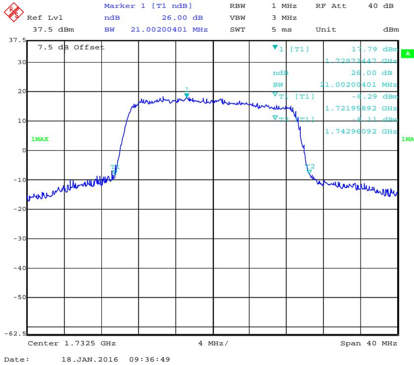
**16-QAM (20.0 MHz) - 26 dB Bandwidth, Middle channel**
