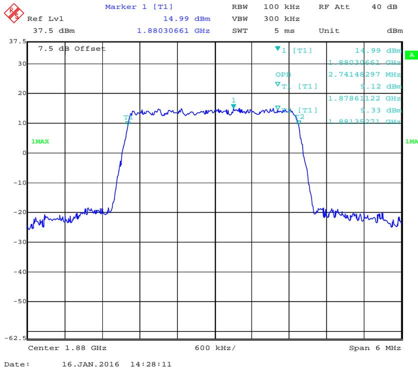
**QPSK (5.0 MHz) - 99% Occupied Bandwidth, Middle channel**
