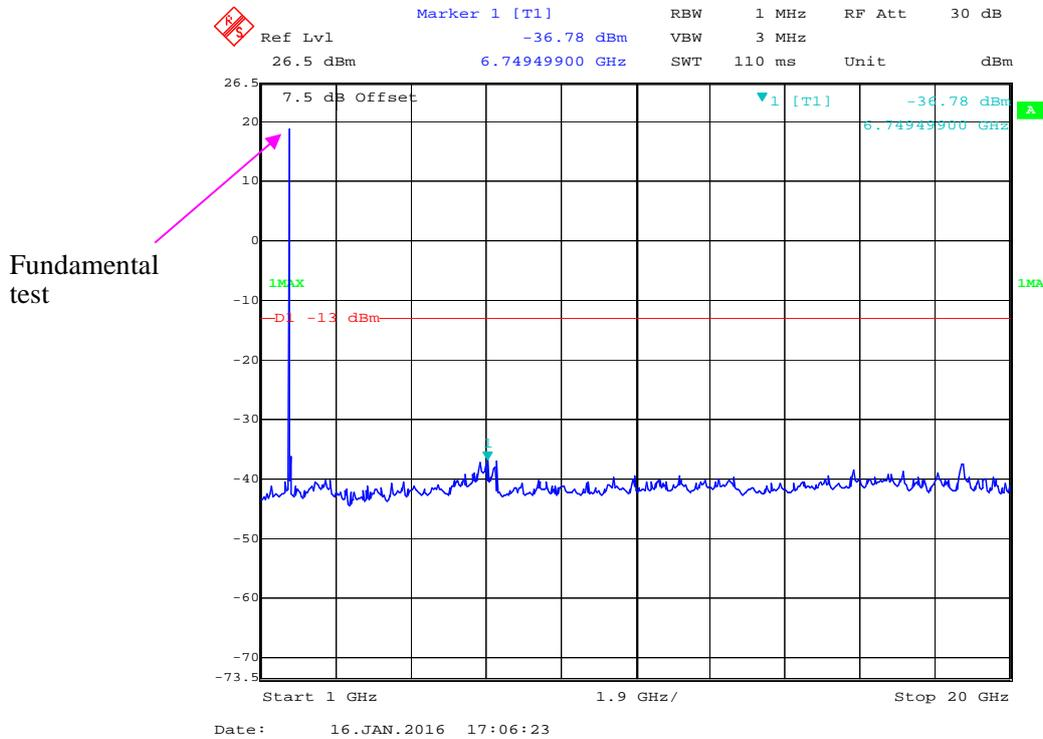
**30 MHz - 1 GHz (10.0 MHz, Middle Channel)**
