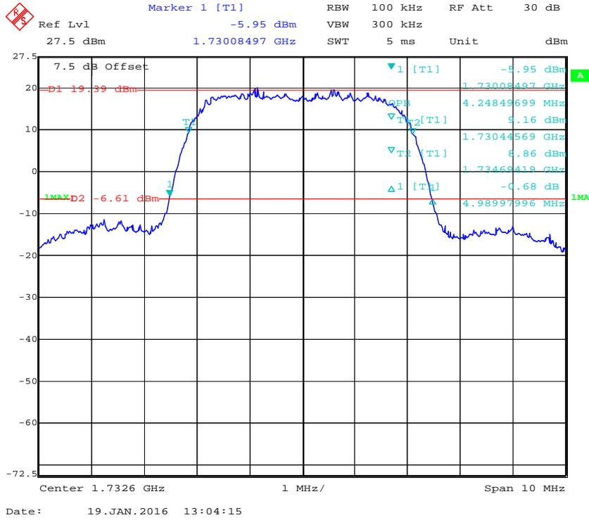
**99% Occupied & 26 dB Emissions Bandwidth for HSUPA (BPSK) Mode**
