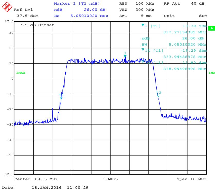
**QPSK (10.0 MHz) - 26 dB Bandwidth, Middle channel**
