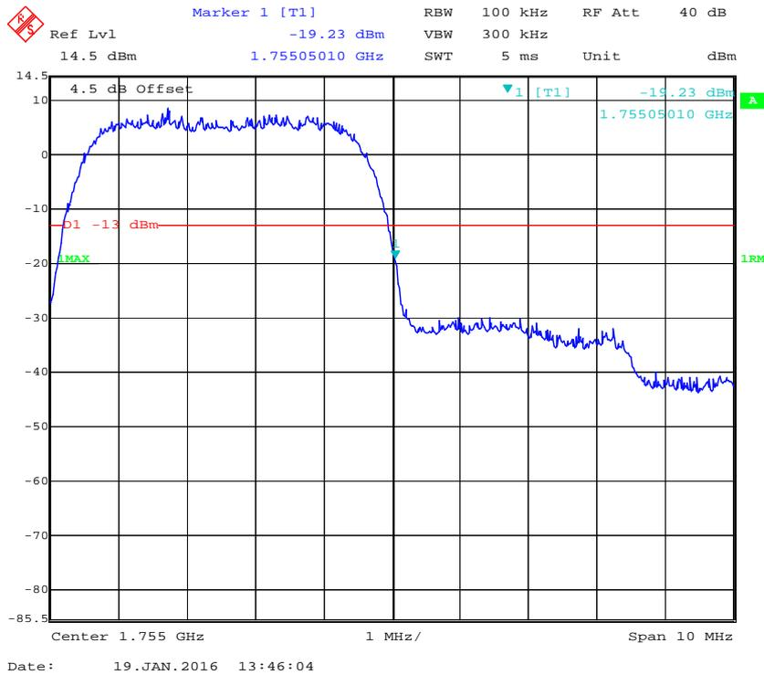
**AWS Band, Left Band Edge for HSUPA (BPSK) Mode**
