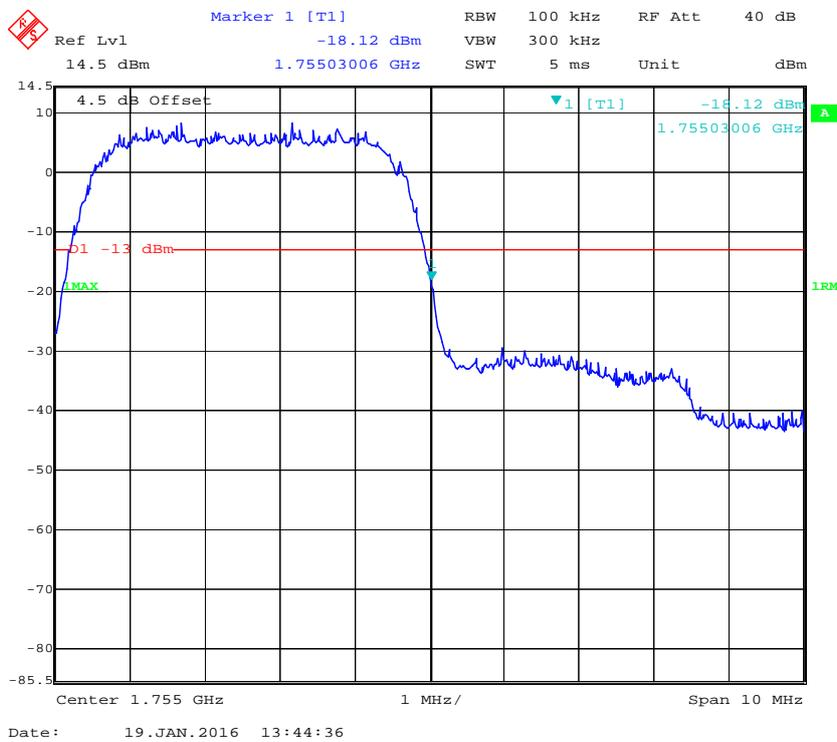
**AWS Band, Left Band Edge for HSDPA (16QAM) Mode**
