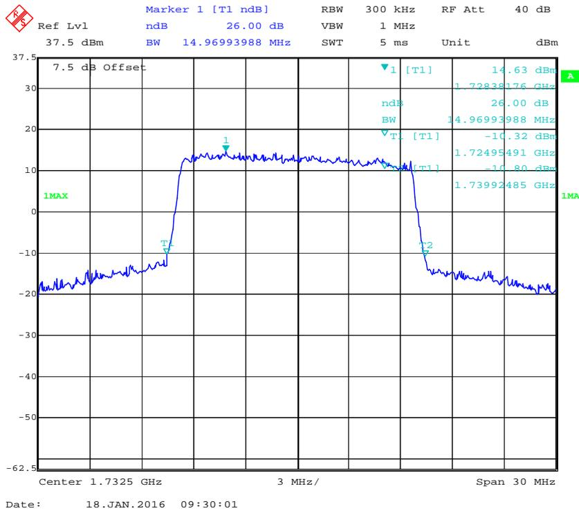
**QPSK (20.0 MHz) - 26 dB Bandwidth, Middle channel**
