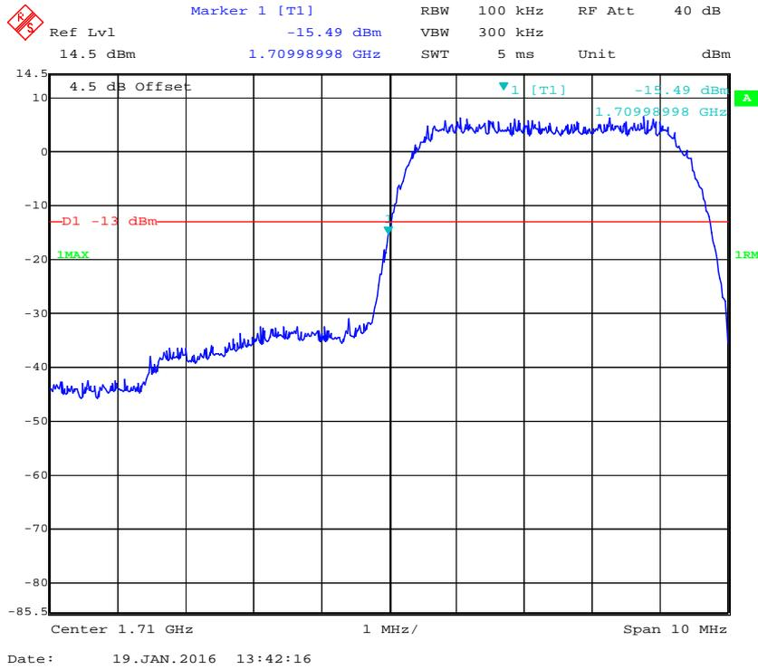
**AWS Band, Right Band Edge for HSDPA (16QAM) Mode**
