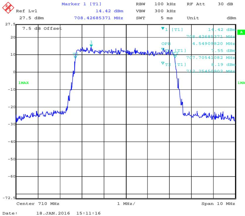
**QPSK (10.0 MHz) - 99% Occupied Bandwidth, Middle channel**
