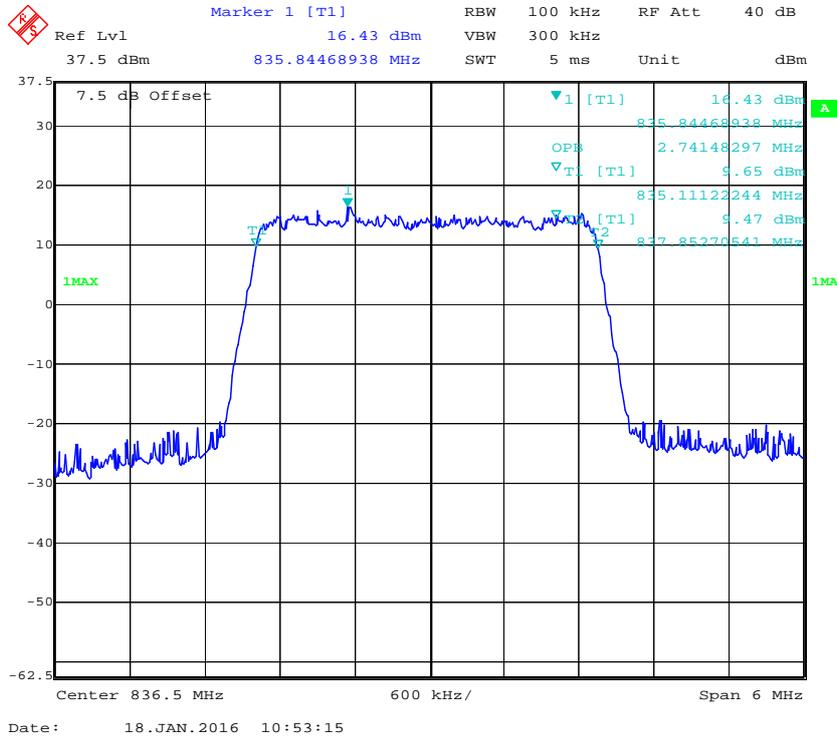
**16-QAM (3.0 MHz) - 99% Occupied Bandwidth, Middle channel**
