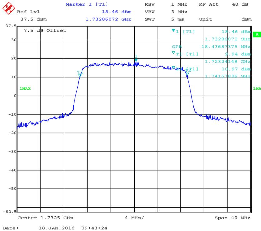
**QPSK (1.4 MHz) - 26 dB Bandwidth, Middle channel**
