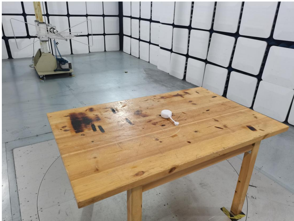
Photo of Radiation Emission Test
