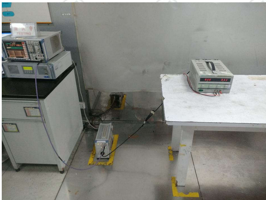
Conducted emissions Test Setup
