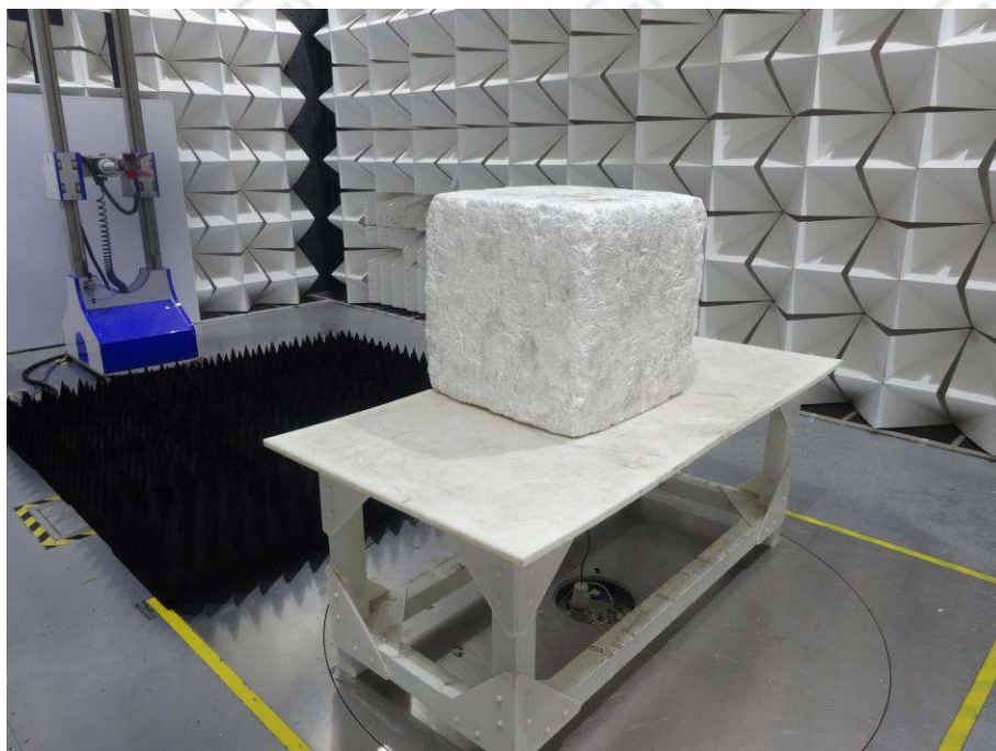
Radiated spurious emission Test Setup-3(Above 1GHz)
