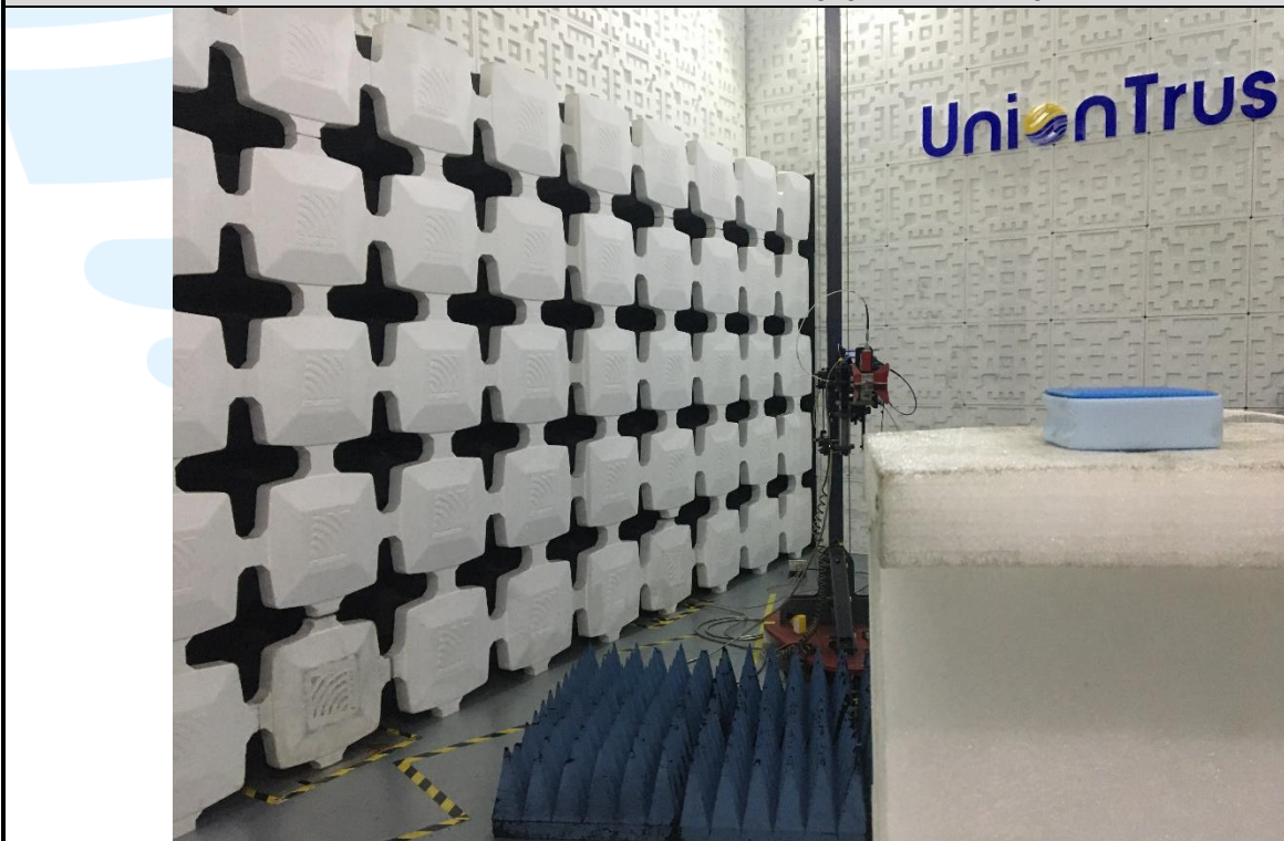
Radiated emission Test Setup (Above 1 GHz)
