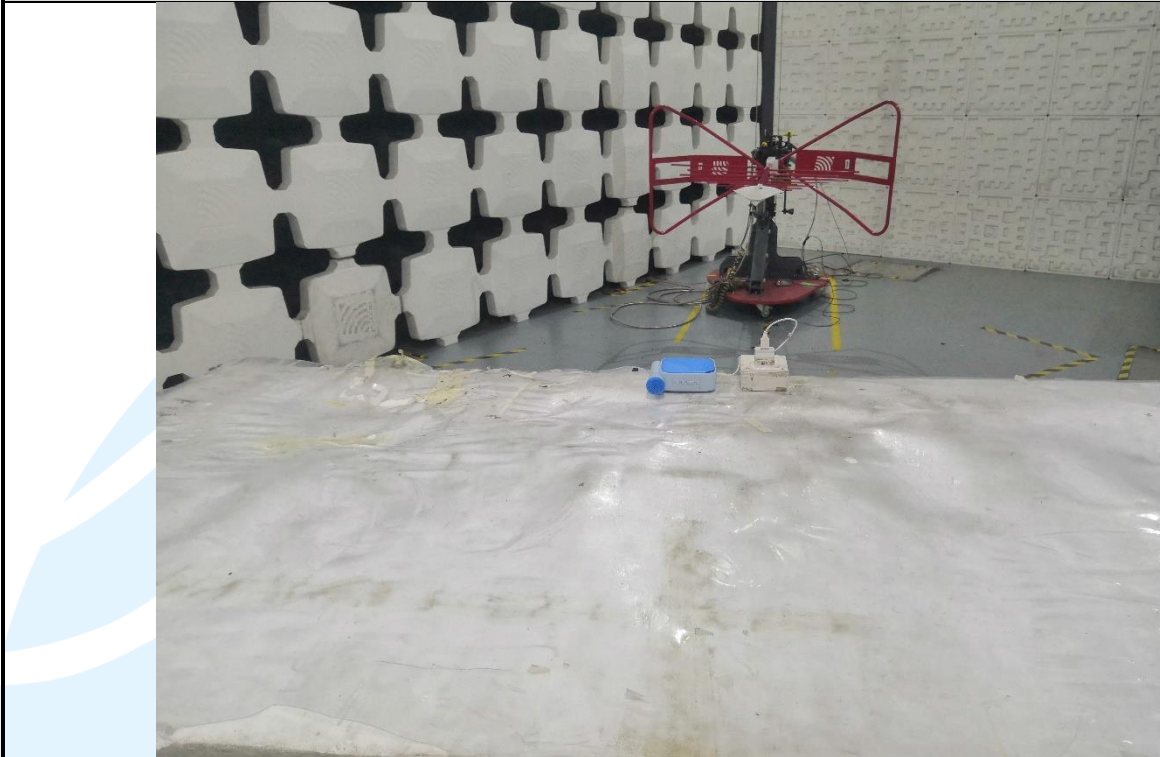
Radiated emission Test Setup (30 MHz~1 GHz)
