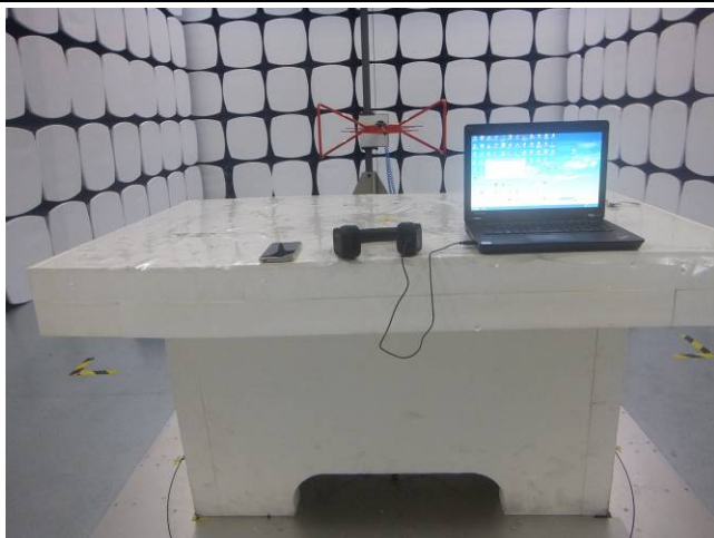
Radiated Spurious Emissions Test Setup Below 1GHz
