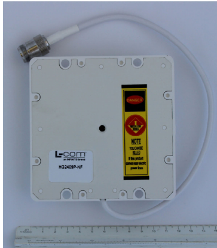
Connector: N-Female on 25cm coax VSWR: <1.5:1 Mount: Mast w/ U-Bolt Kit Vertical 3dB Beamwidth: 65° Horizontal 3dB Beamwidth 75°
