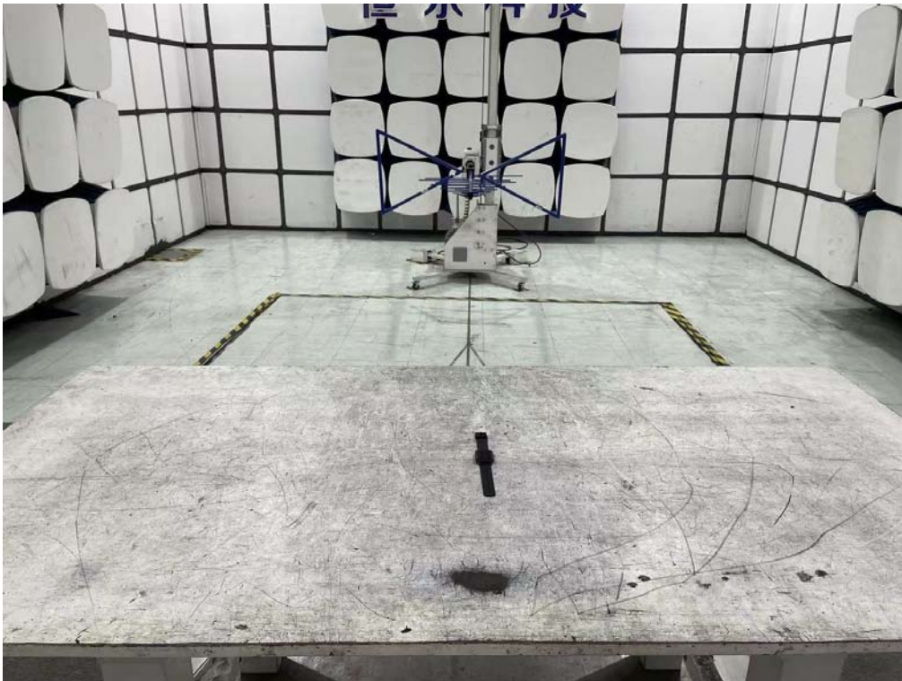
Radiated emission test: Below 1GHz
