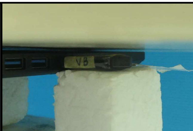
Horizontal Down of EUT Tested at 5 mm
