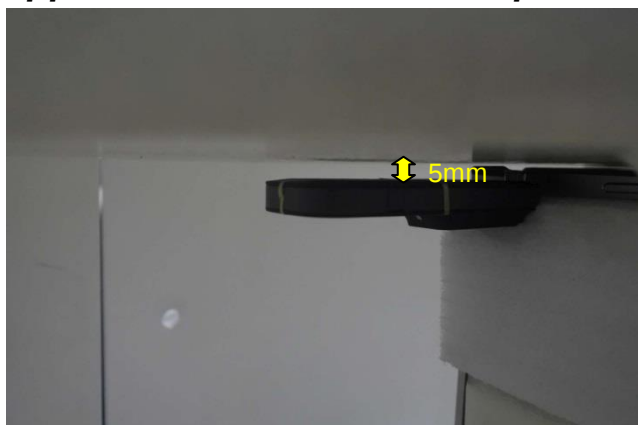
Direct Laptop Plug-in for USB Configuration 1 (Horizontal Up, Test Separation 5 mm)
