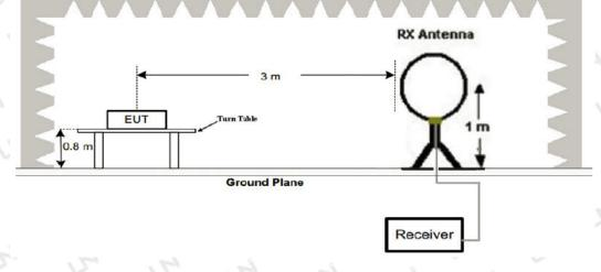
2. Radiated Emission Test-Up Frequency 30MHz~1GHz
