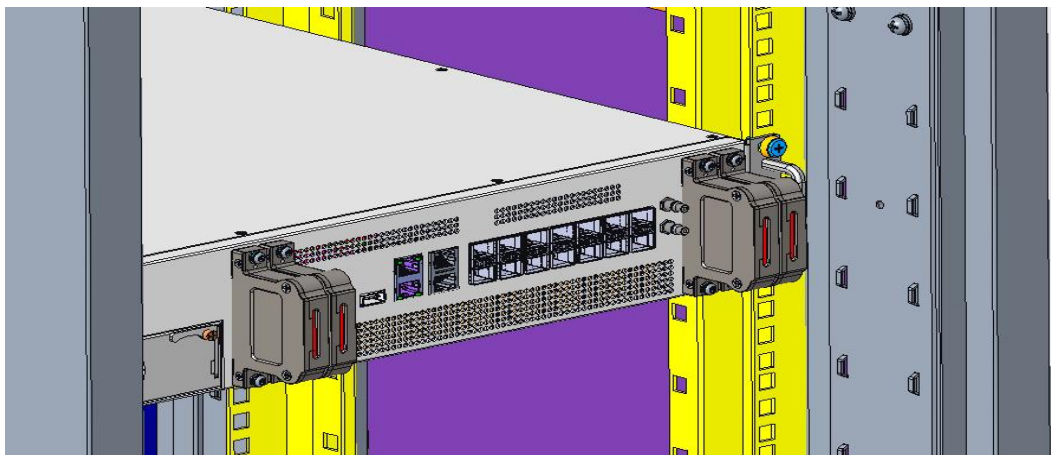
Figure 31 DCU RF cable plug installation
