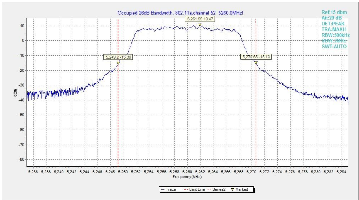
Fig. 4 Occupied 26dB Bandwidth (802.11a, 5260MHz)
