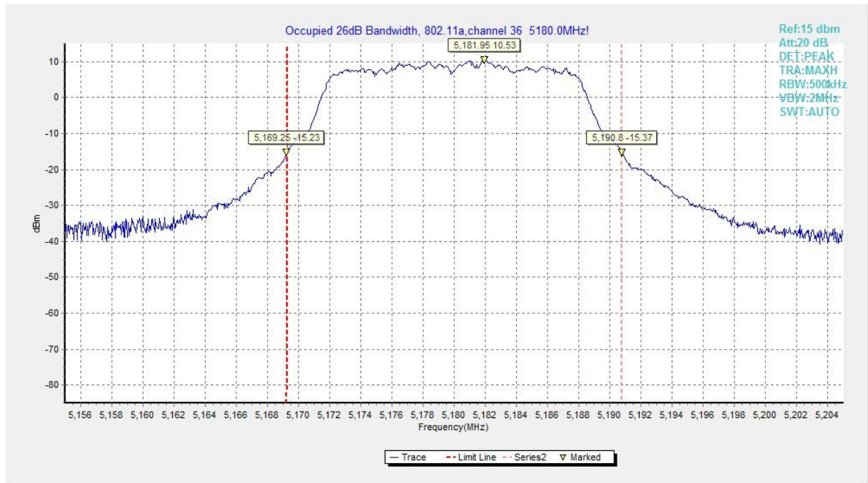
Fig. 1 Occupied 26dB Bandwidth (802.11a, 5180MHz)
