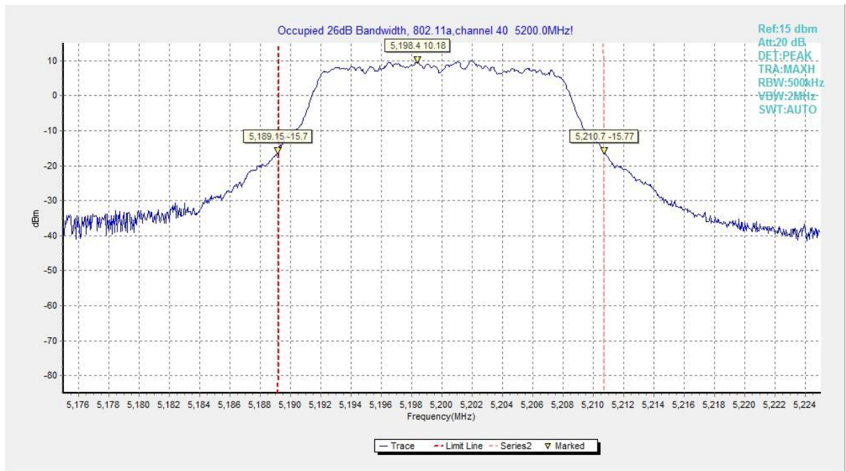
Fig. 2 Occupied 26dB Bandwidth (802.11a, 5200MHz)
