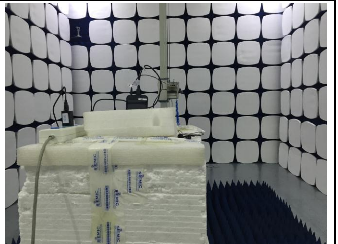
Radiated Spurious Emissions Test Setup Above 1GHz
