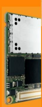
Customers who require a high-quality GSM/GPRS wireless module for their m2m applications but don't need the TC65's Java™ platform should take a close look at the new TC63. Featuring quadband technology, GPRS class 12, and an integrated TCP/IP stack, this module enables GSM/GPRS connectivity of the highest standard.
