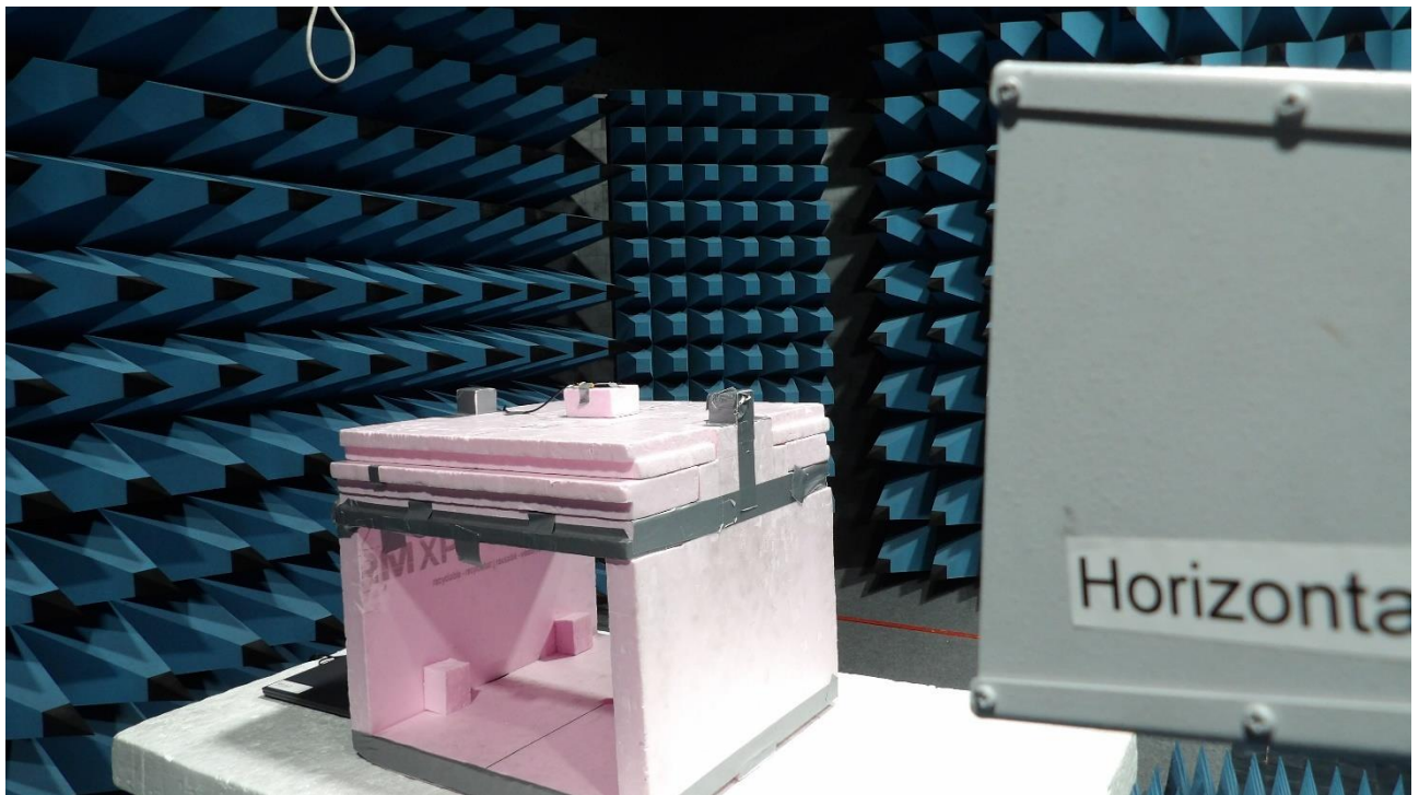
Picture 5: FS-SAC, radiated emission test 1 GHz – 17 GHz (front view)
