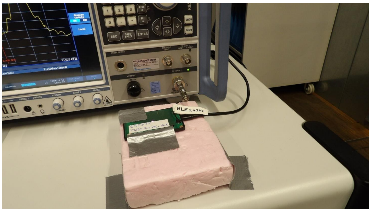
Picture 10: Conducted measurements
