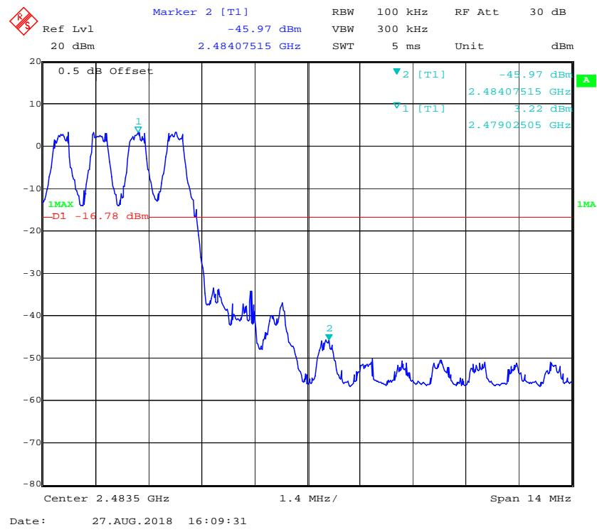
*EDR Mode ( $\pi/4$ -DQPSK):***Band Edge, Left Side**
