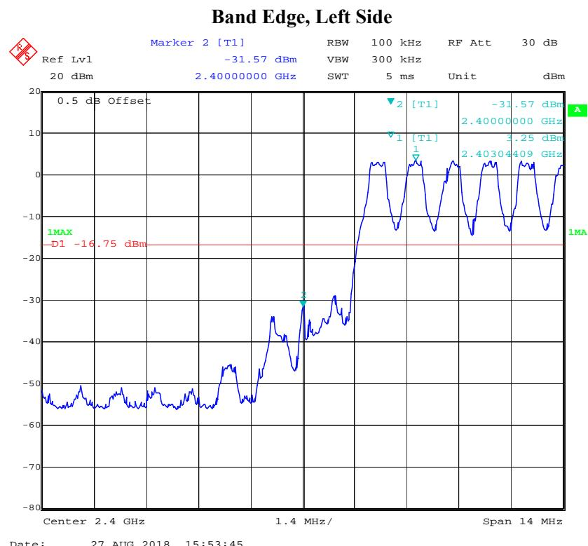
**Band Edge, Right Side**
