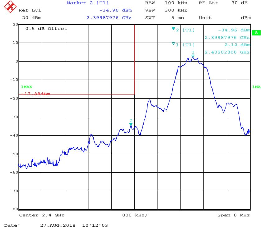
**Band Edge, Right Side**
