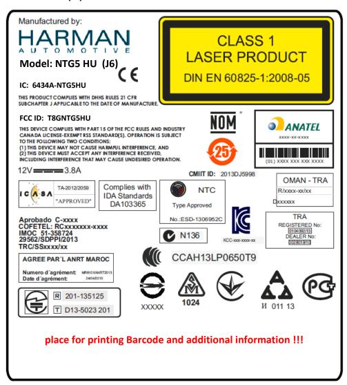
Placement: The Label will be placed on the chassis top (compare picture below)
