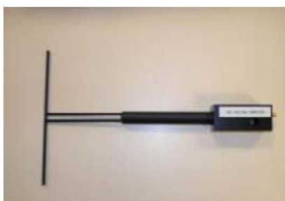
Figure 1 – Satimo COMOSAR Validation Dipole
