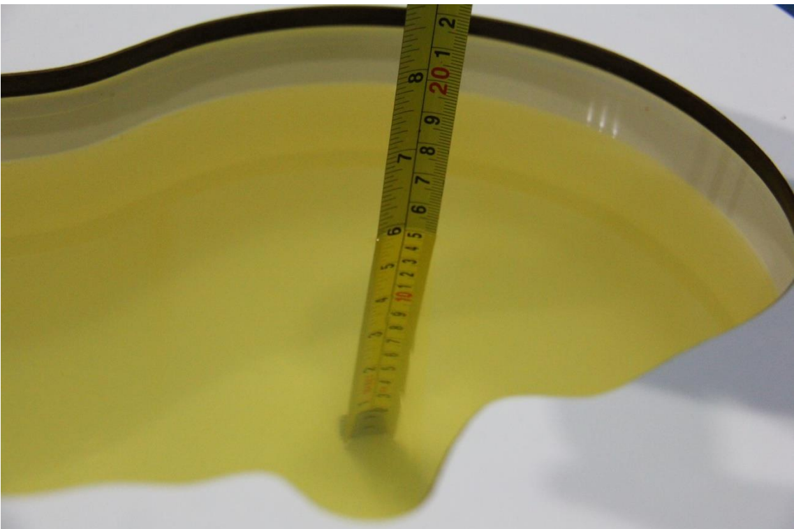
Picture 7-4 Liquid depth in the Head Phantom (1900 MHz)
