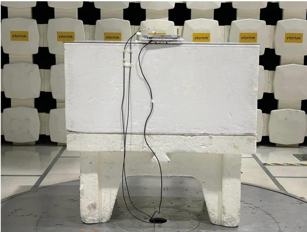
Radiated Emissions Test Setup, 18-40 GHz
