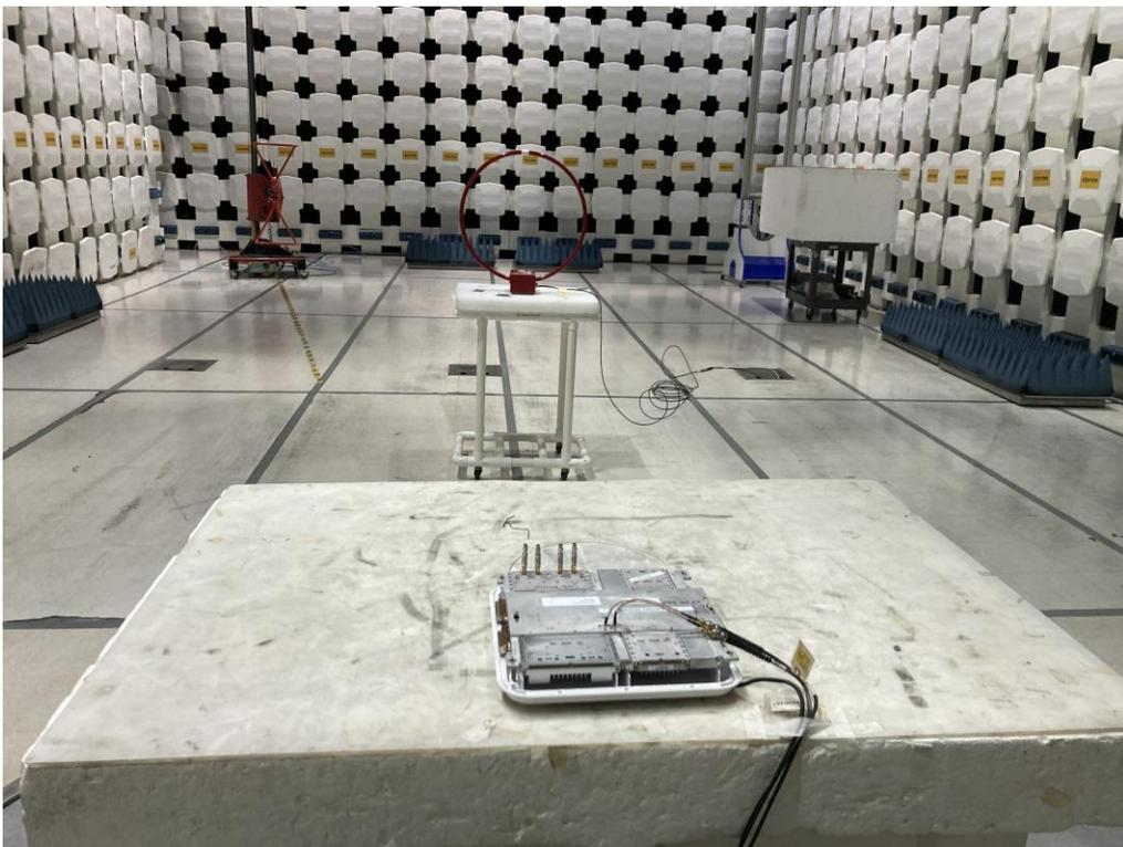
Radiated Emissions Test Setup, 9 kHz – 30 MHz, Y-Axis
