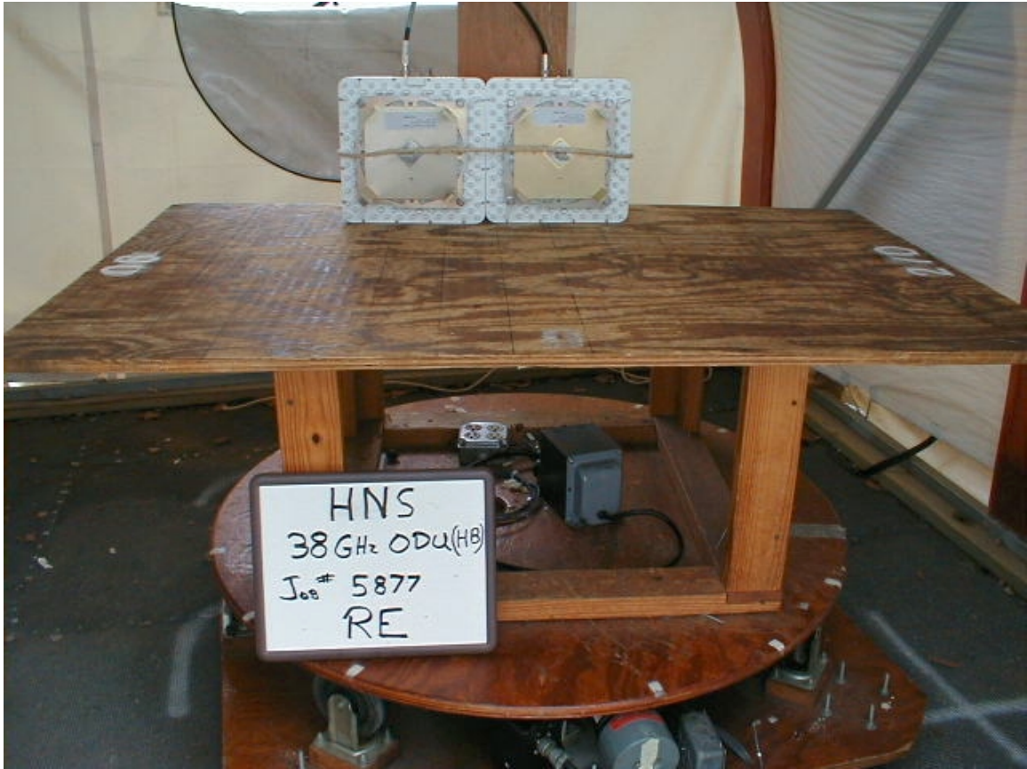
Figure 2: Radiated Emission Test setup (Open Field Site) (30 MHz-18 GHz)
