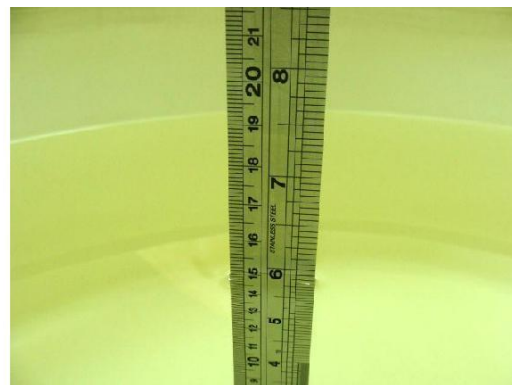
Fig 7.2 Photo of Liquid Height for Body SAR
