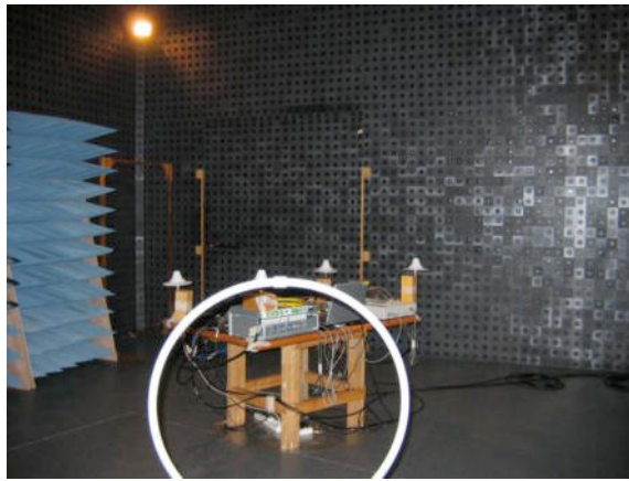
Photograph 1.10.2 Setup for spurious emission field strength measurements from 30 to 1000 MHz
