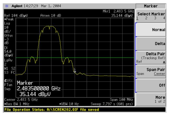
Detector mode: Peak Polarity: Horizontal
