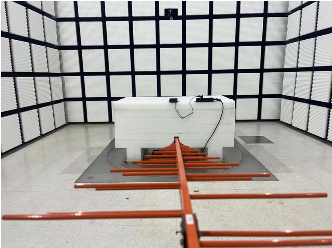
Radiated Emission Below 1GHz rear View
