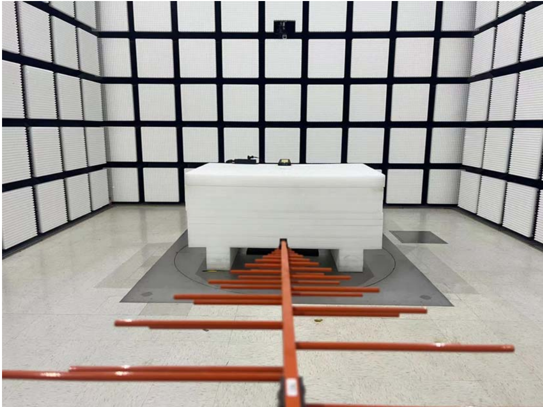
Radiated Emission Below 1GHz rear View
