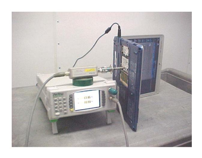
Maximum Peak Output Power Measurement Setup
