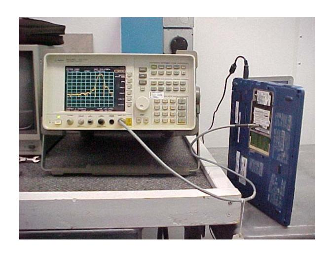
Conducted Emissions at Antenna Terminal Setup
