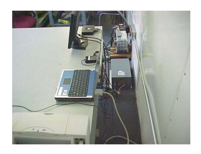
AC Conducted Emissions Measurement (Rear View) Setup
