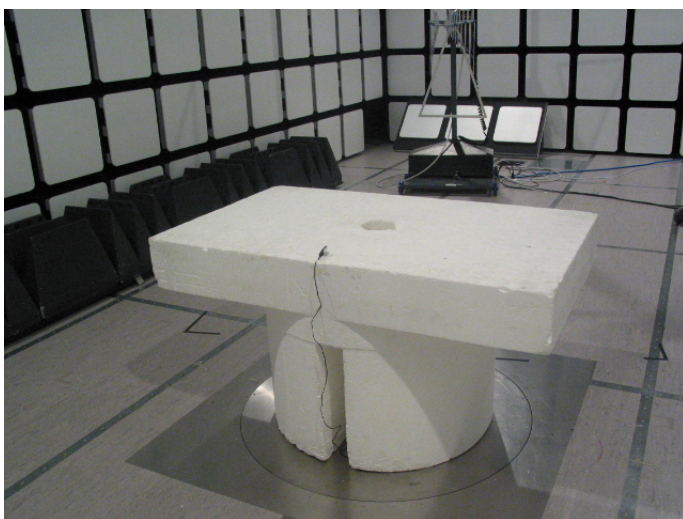
Picture 2 Radiated emission measurement Bluetooth TX
