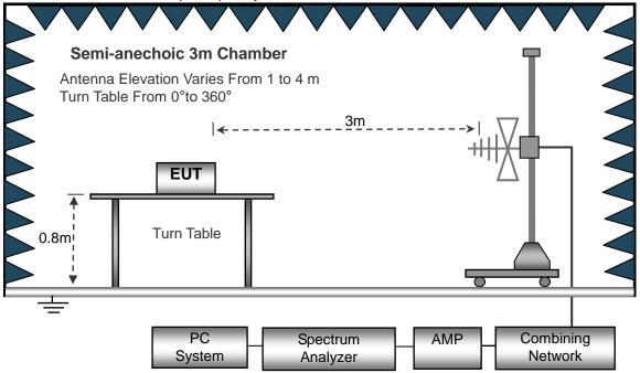
(C) Radiated Emission Test-Up Frequency Above 1GHz
