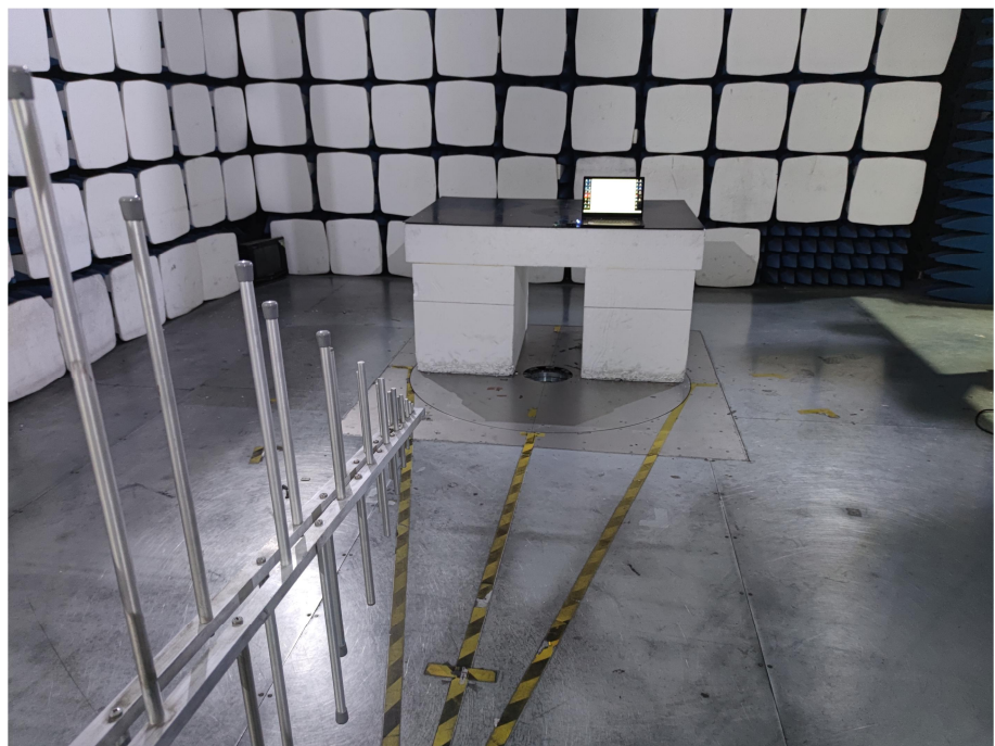
Radiation Emission Test Setup (30MHz to 1GHz)
