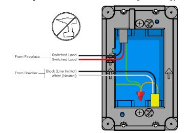
Identify and connect the wires to the back of the fireplace switch. Insert the wire into the terminal and secure it by hand-tightening the set screw.
