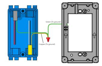
Using a manual screwdriver, install the mounting plate to the wall box. **Do not**overtighten the screws. Pull the rest of the wires through the mounting plate.
