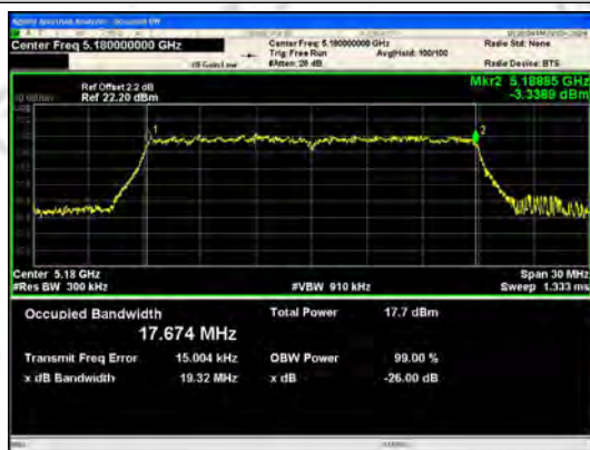
IEEE 802.11ac_Channel 36_20MHz_Antenna 1
