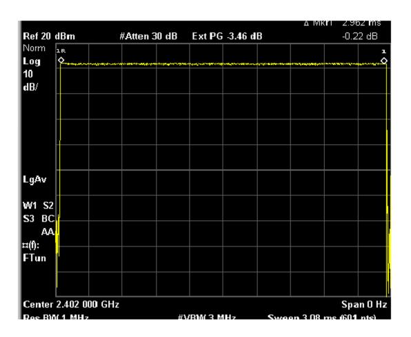
Plot Showing numbers of pulses in 1 second in DH5 Mode: 4 peaks of DH5 packets in 1 second
