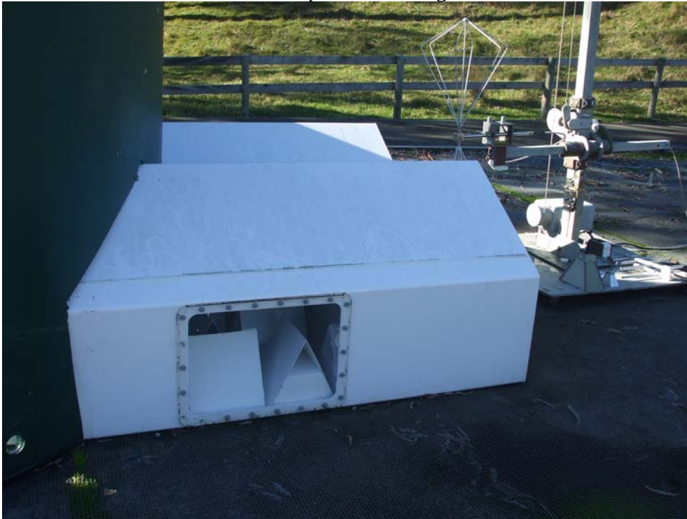
Cone enclosure up close showing the cones
