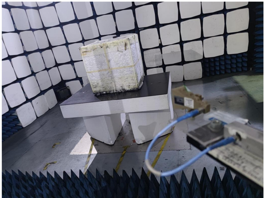
Radiation Emission Test Setup (Above18GHz)
