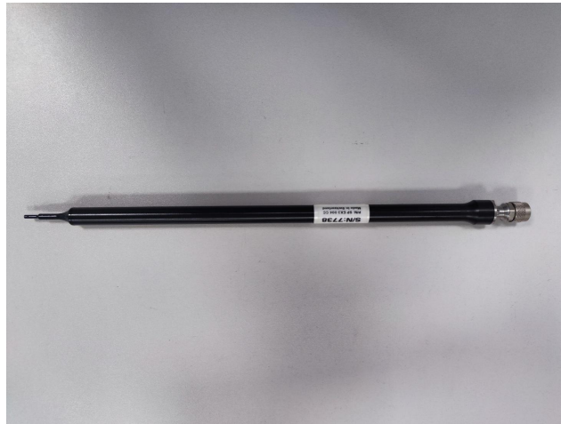
Figure 1-Speag COMOSAR Dosimetric E field Dipole
