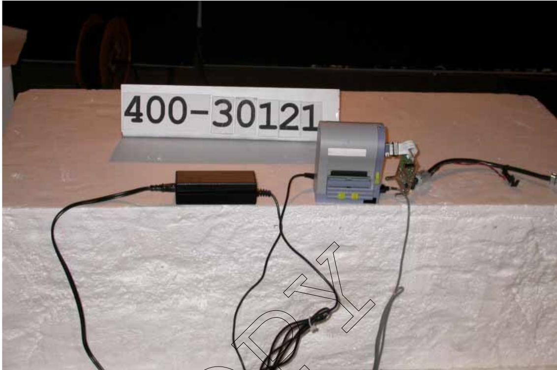
**PHOTOGRAPHS OF EUT CONFIGURATION FOR AC POWER LINE CONDUCTED EMISSIONS MEASUREMENT**
