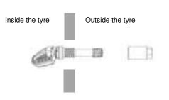
1.4 Place nut<sup>®</sup> on the valve stem, and tighten with 5 Nm (44 inch pounds) torque.
