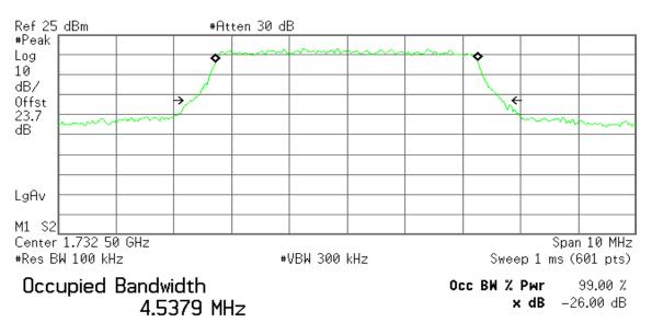
Transmit Freq Error -9.866 kHz x dB Bandwidth 5.348 MHz
