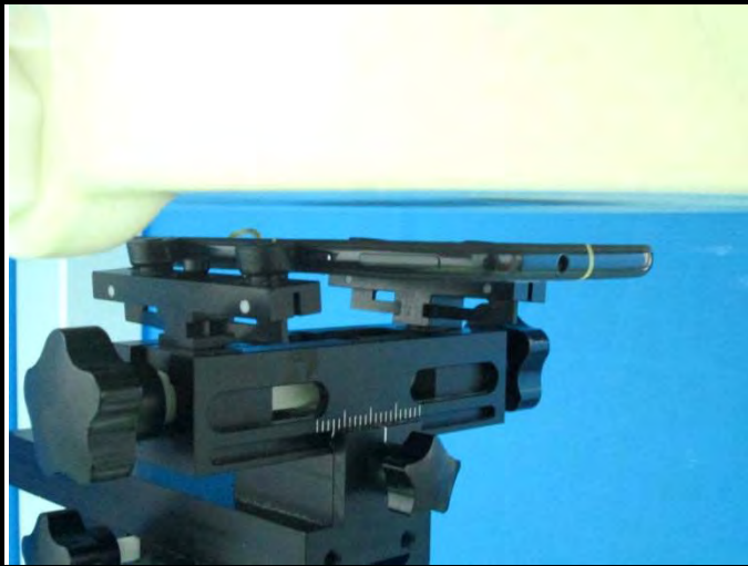
Front Face of EUT with 1.0 cm Gap
