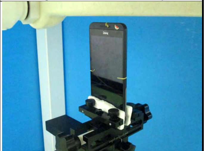
Bottom Side of EUT with 1.0 cm Gap
