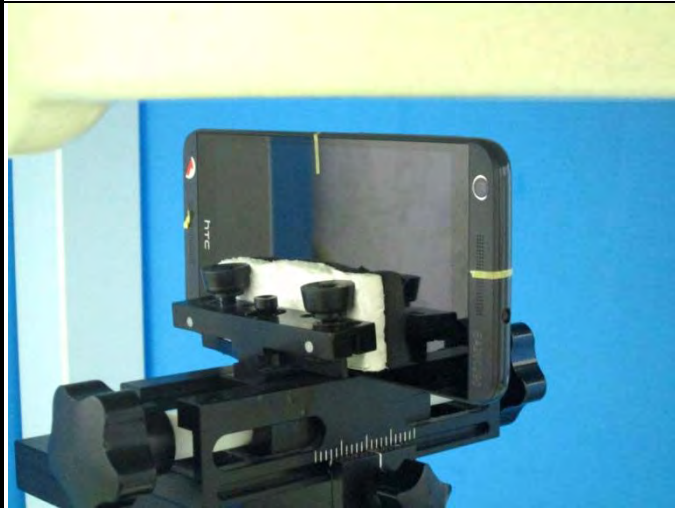
Left Side of EUT with 1.0 cm Gap
