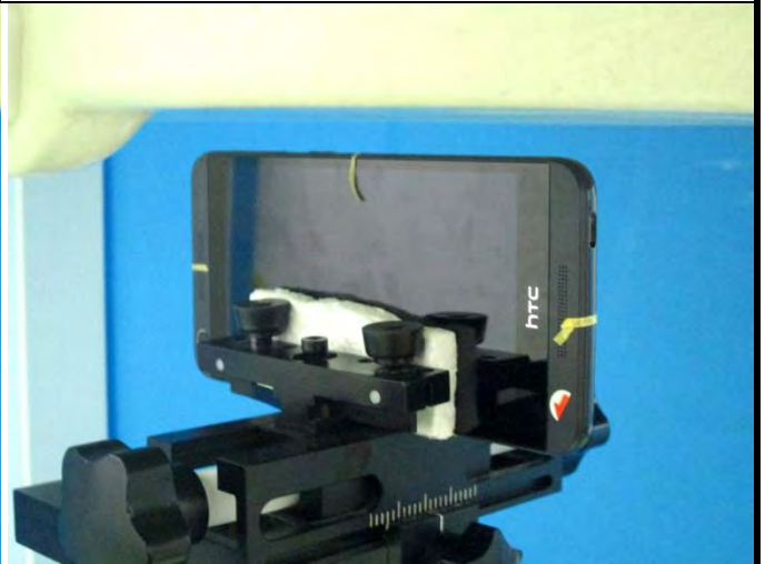
Right Side of EUT with 1.0 cm Gap
